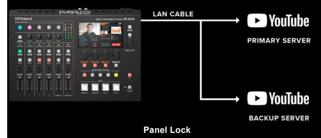
Panel Lock prevents users from accidentally changing settings that could disrupt a broadcast. You can disable access to a wide range of hardware controls and menu parameters on an individual basis, leaving only the essential functions needed for the livestream.
